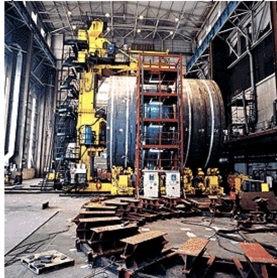
Fig.2 - Rotated circumferential submerged arc welding shop.
