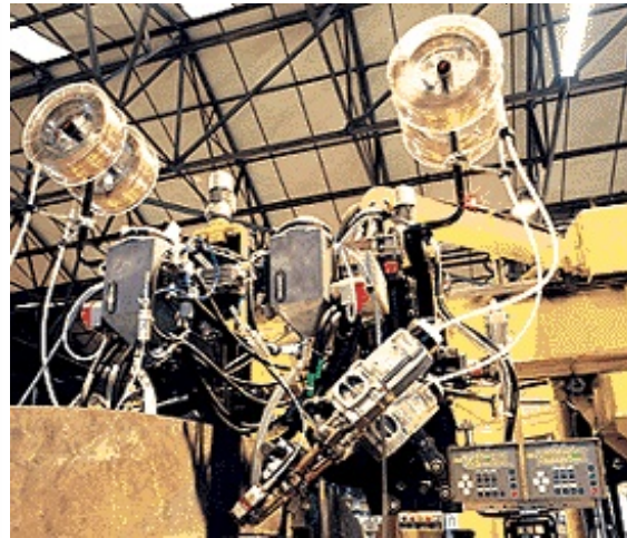
Fig.1 - The twin tandem submerged arc (SA) arrangement for joining the frame web to table joints.
