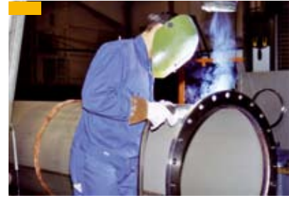
Manual MAG welding of a welded flange
