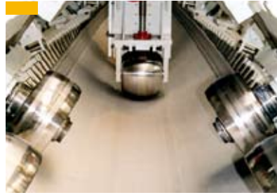
Continuous production of pipes from coil
